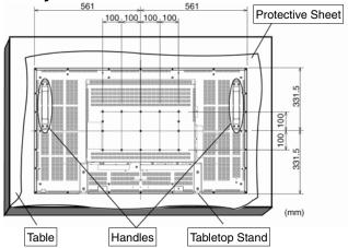
Lay the protective sheet on a table, which was wrapped around the monitor when it was packaged, beneath the screen surface so as not to scratch the screen face.
